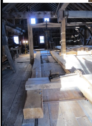
Left: The carriage is in place, next the construction of the Head and Tailstocks with its screw works that will adjust the log on the carriage for each cut.
