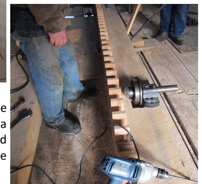
Left: The carriage is in place, next the construction of the Head and Tailstocks with its screw works that will adjust the log on the carriage for each cut.
